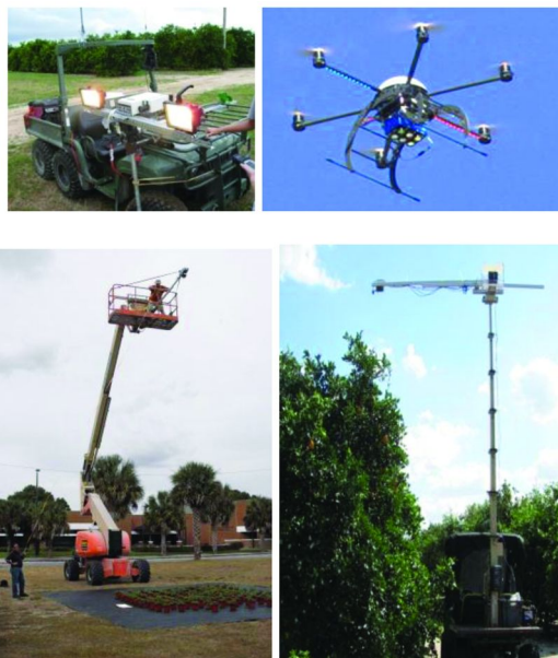
Figure 1. Sensor platforms. (a) Sensors mounted in front of a utility vehicle, (b) sensors mounted on a retractable mast connected to an agricultural vehicle, (c) high-lift platforms attached to a vehicle, and (d) unmanned aerial vehicle (not to scale). [Source: Reza Ehsani]
